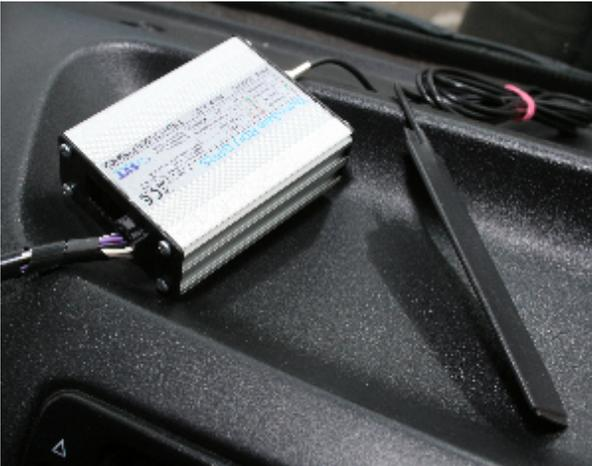
"TachoSafe Remote Download GPRS" downloads remotely the digital tachograph. The remote download unit (RDU) is permanently installed on the truck and it is connected to the digital tachograph. The downloads are initiated manually or by a scheduler through an application installed on PC. The system works in the background but it warns the user in case of errors.
