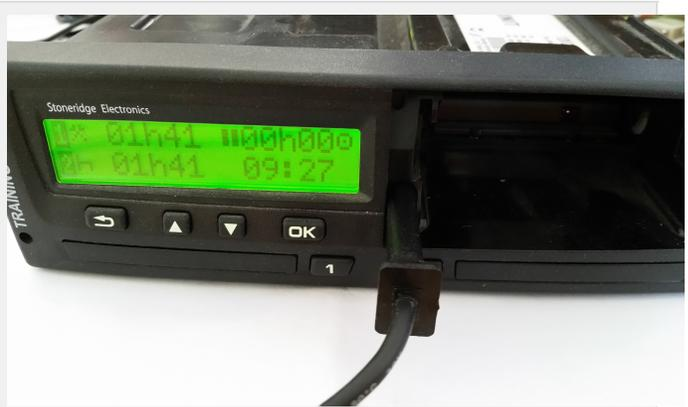
Front download cable connected to tachograph
